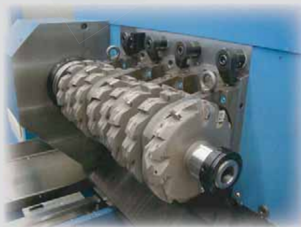
Fraisage culasse Nockenwellenkasten Milling cylinder head
